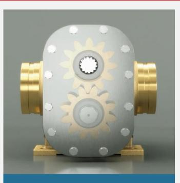
A gear pump uses internal gears to grab the concentrate. The advantages of using gear pumps are that flow is not pulsating, and the pump "grip" very well both high and very high viscosity concentrates.
