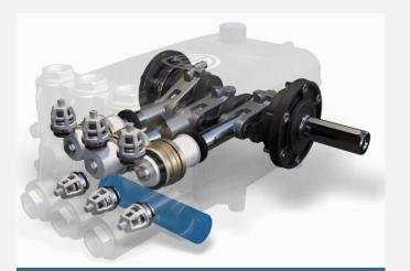
Piston Pumps (-PP) is a reciprocating pump and perform at their best at low to medium viscosities due to the Piston pump principle; for each revolution, the plunger sucks concentrate and then presses it out - the concentrate goes from zero to full speed twice per revolution.
